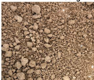
Figure 5. Granulation and Drying of NPK 6:12:24 + 6% S Samples (Before Sieving)
