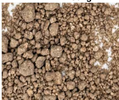
Figure 5. Granulation and Drying of NPK 6:12:24 + 6% S Samples (Before Sieving)
