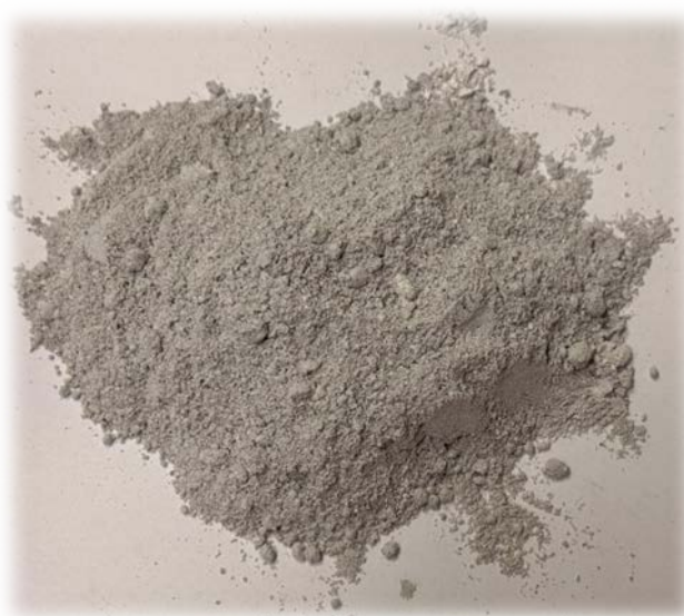
Figure 3. Ash Obtained from the Combustion of Sunflower Husks
